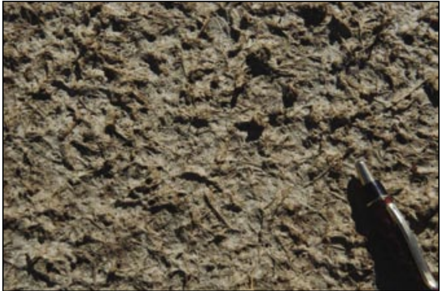
Figure 4—Hydromulch fibers form a smooth dense mat.
