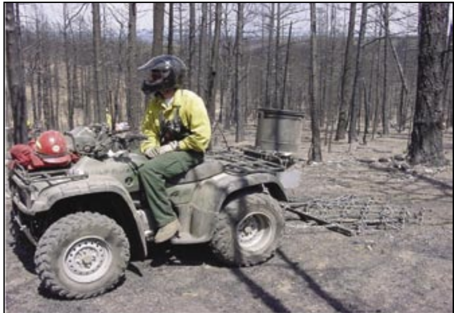
Figure 39—Use of an ATV and a chain harrow to scarify and seed soils.
